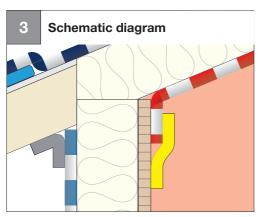
• Vapour control layer joined to timber wall with Sicrall
