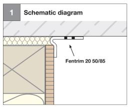
Joining timber wall construction to non-plastered masonry or concrete
