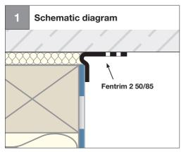
Joining facade membrane to nonplastered masonry or concrete
